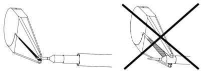
Spring loaded probe tips offer a method of probing signals that is less susceptible to vibration or movement than traditional rigid tips. Many users find it easier to use this type of tip. The spring loaded tips work when they are either partially or fully compressed and are protected against over compression damage.
