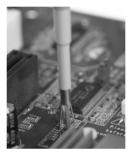
The recommended PCB layout is shown in the manual that accompanied your N2870A Series probe. The PCB socket is compatible with hand soldering and reflow processes. After soldering the socket - both the signal contact and ground contact - to the board, simply insert the probe. The PCB adapter is compatible with either the rigid or spring-loaded probe tip.
